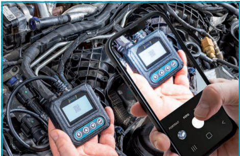
Generation of QR codes for sharing the test results on a smartphone/tablet
