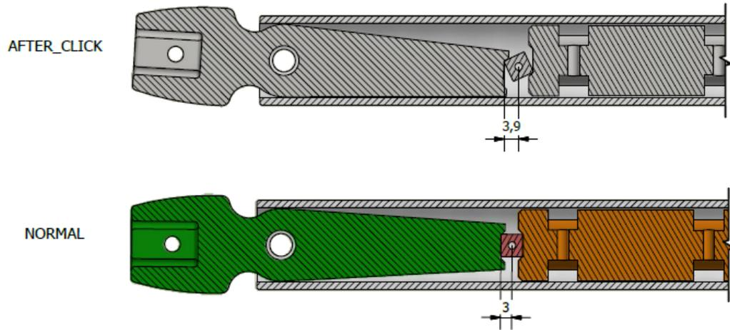
This conception of click mechanism is based on the friction of the square parts. After each tightening, the geometry of the parts change a little due to the mechanical wear and oblige the customer to adjust the spring to maintain the same level of torque
