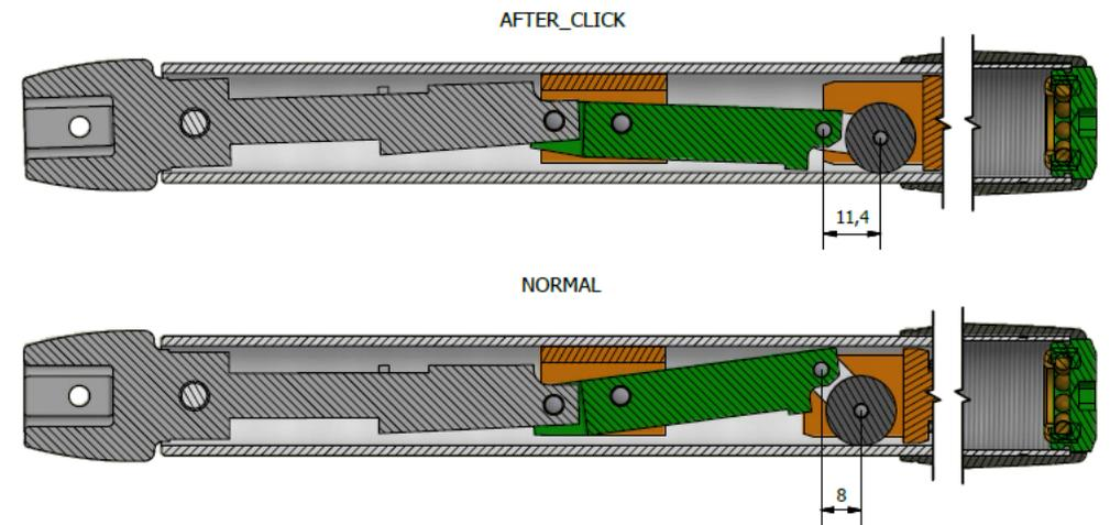
This conception of click mechanism reduce at the minimum the friction and the mechanical wear and authorize the customer to use the wrench without any adjustment with the same quality of tightening.
